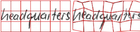
Fig. 3. Word image with uniform grid superimposed. 2nd image (right) with distorted grid and image distorted accordingly.
